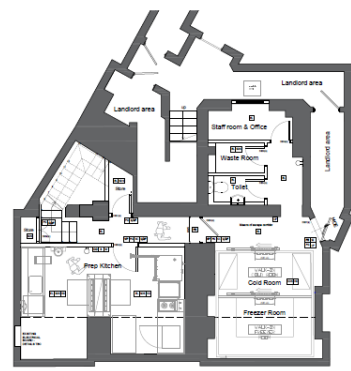
2 Proposed Basement Plan Scale: 1:500
